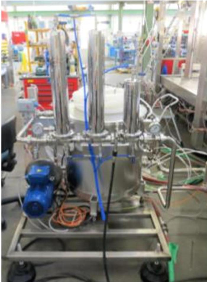
Water microfiltration from inside the bottles washing water
